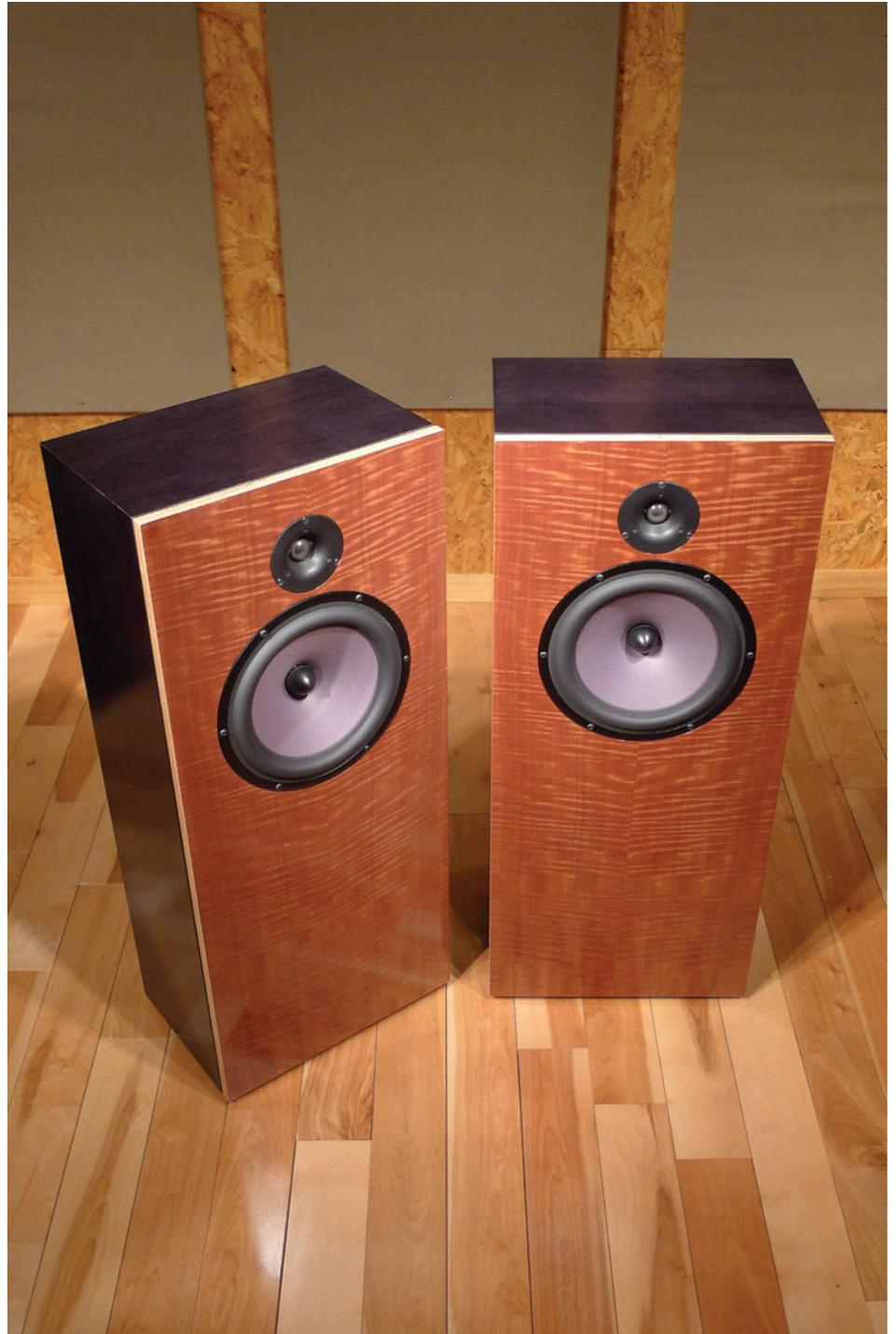
generous, 250 mm mid/bass driver featuring an untreated paper cone and a phase plug. The driver is a bespoke design, manufactured to Devore's specifications, and is partnered by a twin-magnet, horn-loaded 25 mm silk dome tweeter. The crossover point appears to be in the 2 kHz region.
