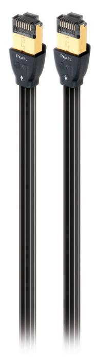
Both Audioquest Ethernet cables under review here conform to the Cat7 standard, which ups bandwidth to 600 MHz, and specifies shielding of individual twisted pairs, as well as for the cable as a whole. The construction provides for four pairs of twisted wire, typically using copperstranded conductors.
